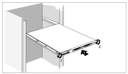
Figure 26: Installing the server
